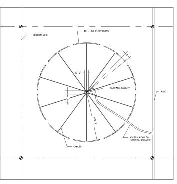
Typical site plan for a ground electrode facility (About 3,000 to 5,000 feet in diameter)
