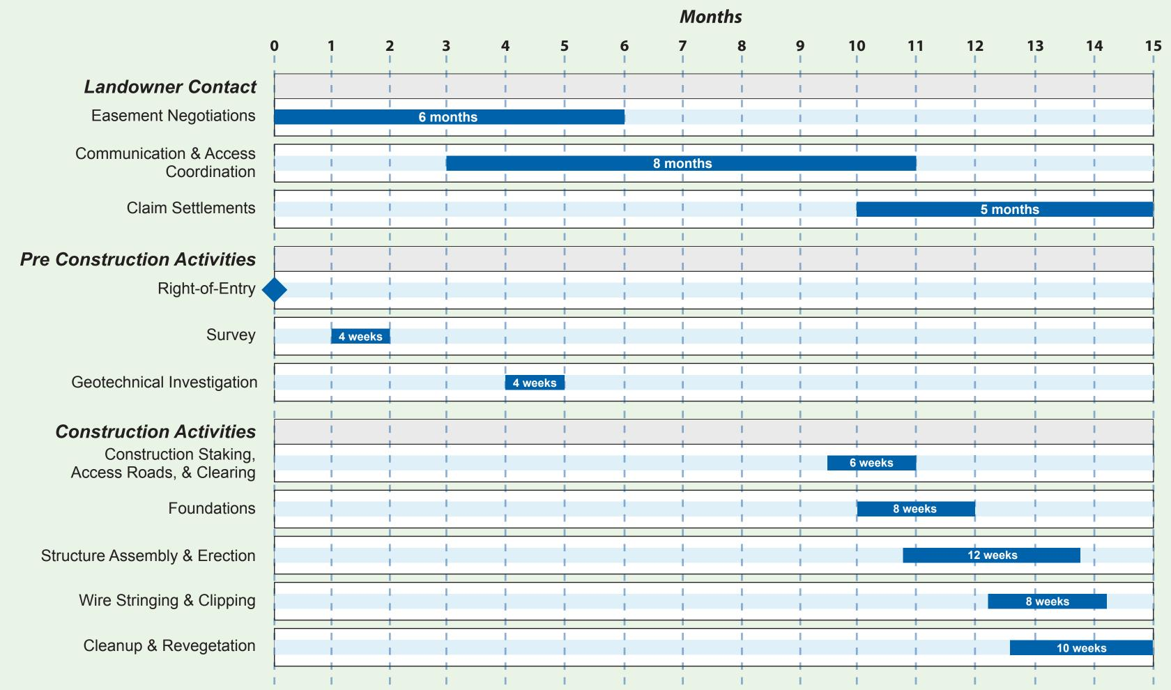
Building a transmission line section requires multiple steps, which are shown in this chart along with the approximate time it takes to complete each step along a typical 50-mile segment. The final sequence and activity durations may vary.
